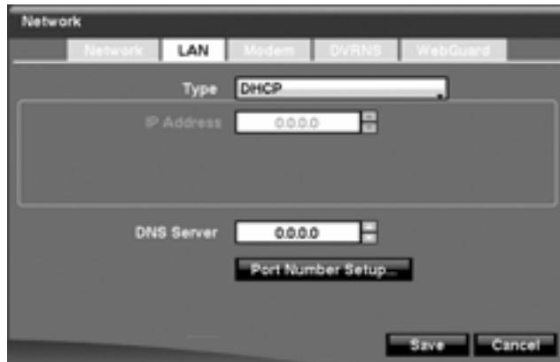
Figure 3-27 LAN (DHCP) Setup Screen
